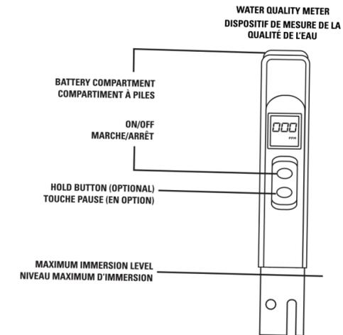
**FOR WATER QUALITY METER:** Remove cap, turn on, submerge in water, change filter when it reads **006 or higher.**
