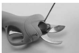
1. Unscrew the screws with a screwdriver and open the lid.
