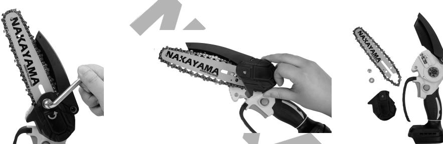
1) Loosen the screw by rotating it counterclockwise with a wrench.
